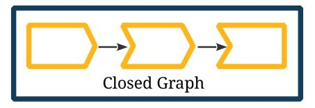
While building a stream, the stream may change shape during its construction. For example, a publisher may be collected into a List of elements. When this happens, the stream becomes a closed graph, since there is no longer an outlet, but just a result, the result being the List of elements:
