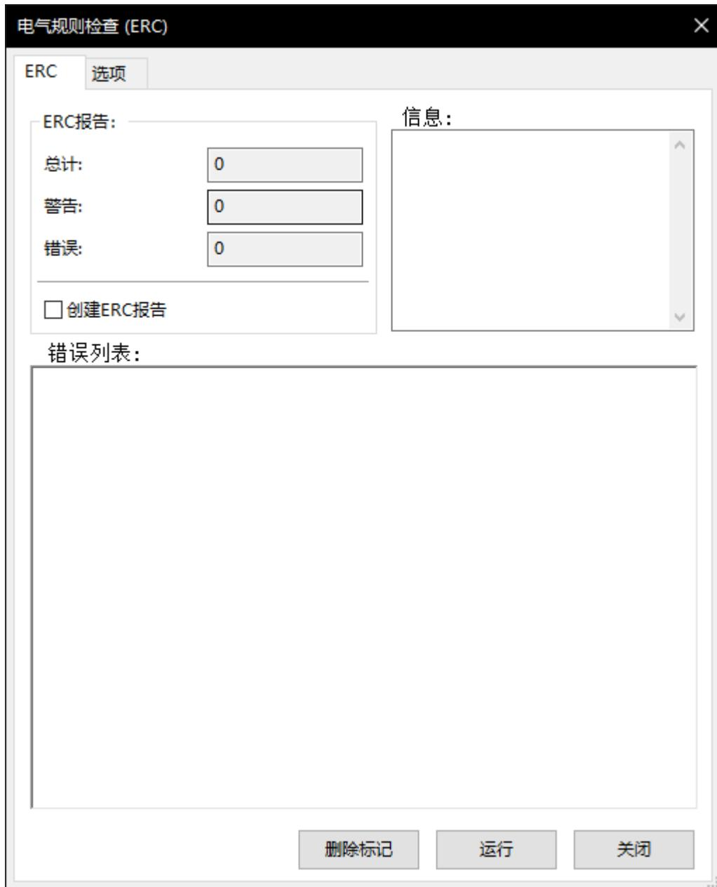
Any warnings or errors are reported in the **Violations** tab, and markers for each violation are placed in the schematic so that they point to the relevant part of the schematic. Warnings are indicated by yellow arrows, and errors have red arrows. Excluded violations are shown as green arrows.
