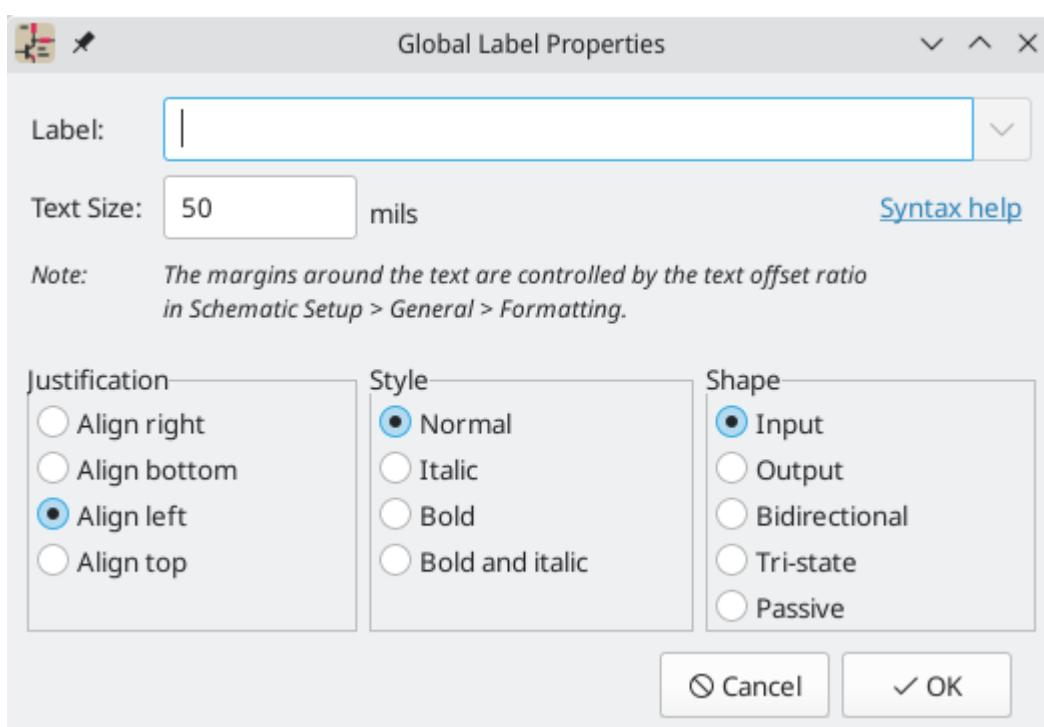
The **Label** field sets the label's text, which determines the net that the label assigns to its attached wire. Label text supports [markup](#) for overbars, subscripts, etc., as well as [variable substitution](#). Use the [Syntax help](#) link in the dialog for a summary.
