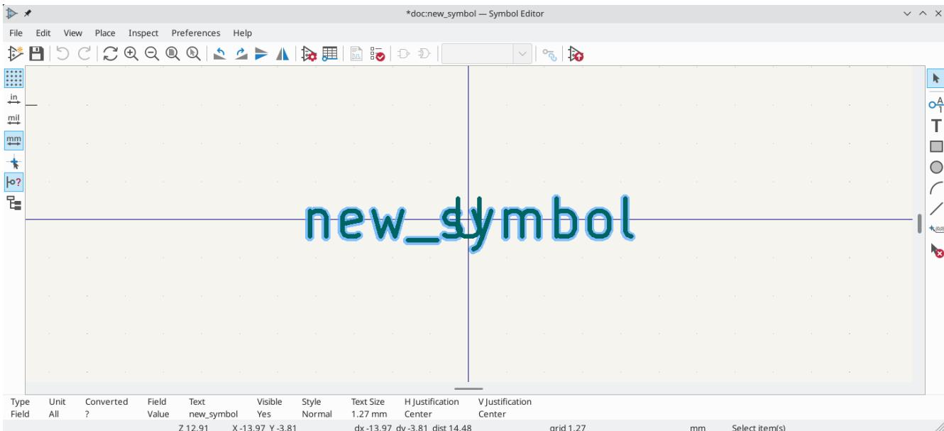
The blue cross in the center is the symbol anchor, which specifies the symbol origin i.e. the coordinates (0, 0). The anchor can be repositioned by selecting the icon and clicking on the new desired anchor position.
