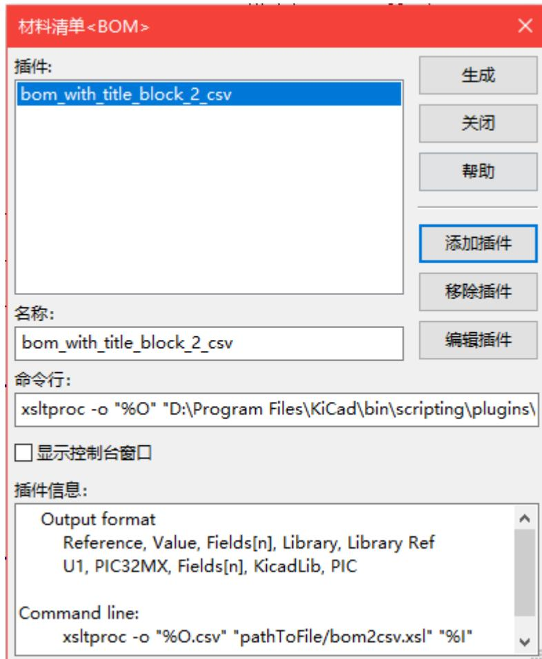
The BOM tool uses an external script to process the design information into the desired output format. Several BOM generator scripts are included with KiCad, and users can also create their own. BOM generator scripts generally use Python or XSLT, but other tools can be used as long as you can specify a **command line** for KiCad to execute when running the generator.
