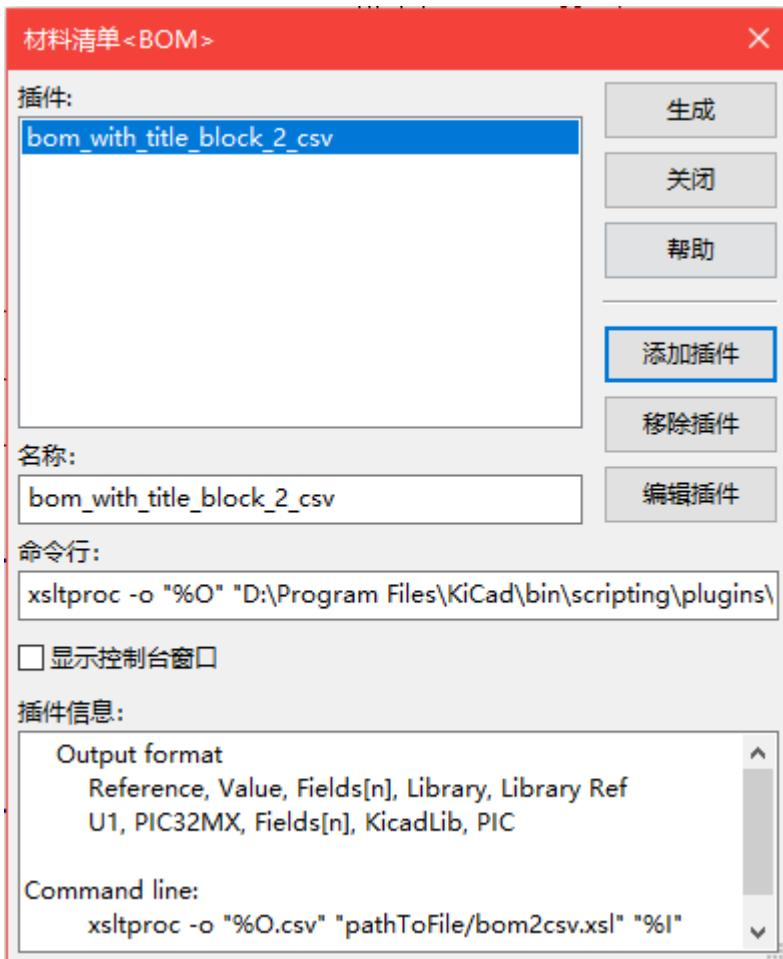
Additional scripts can be added to the list of BOM generator scripts by clicking the button. Scripts can be removed by clicking the button. The button opens the selected script in a text editor.
