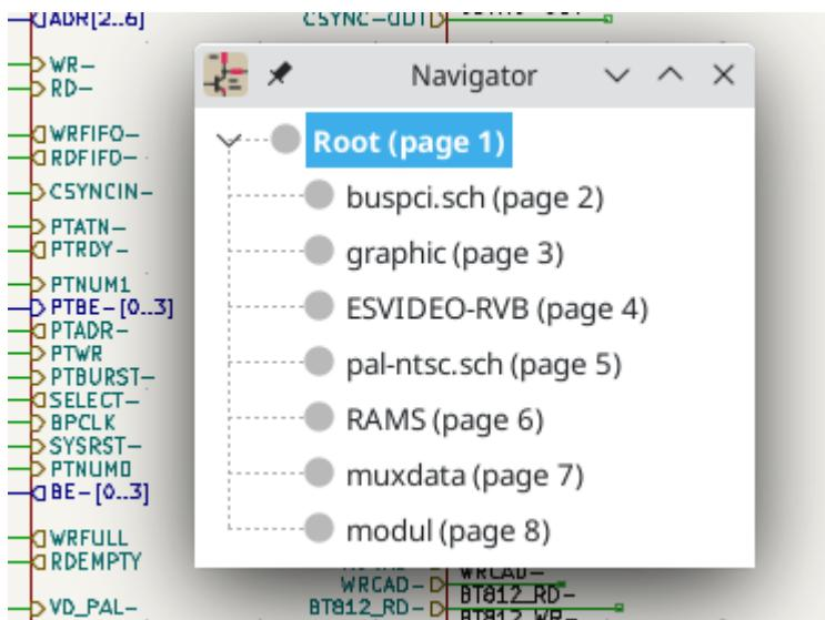
By default, the hierarchy navigator closes after a new sheet is opened. It can be configured to always remain open by selecting the **Keep hierarchy navigator open** option in the Editing Options section of the Schematic Editor preferences.
