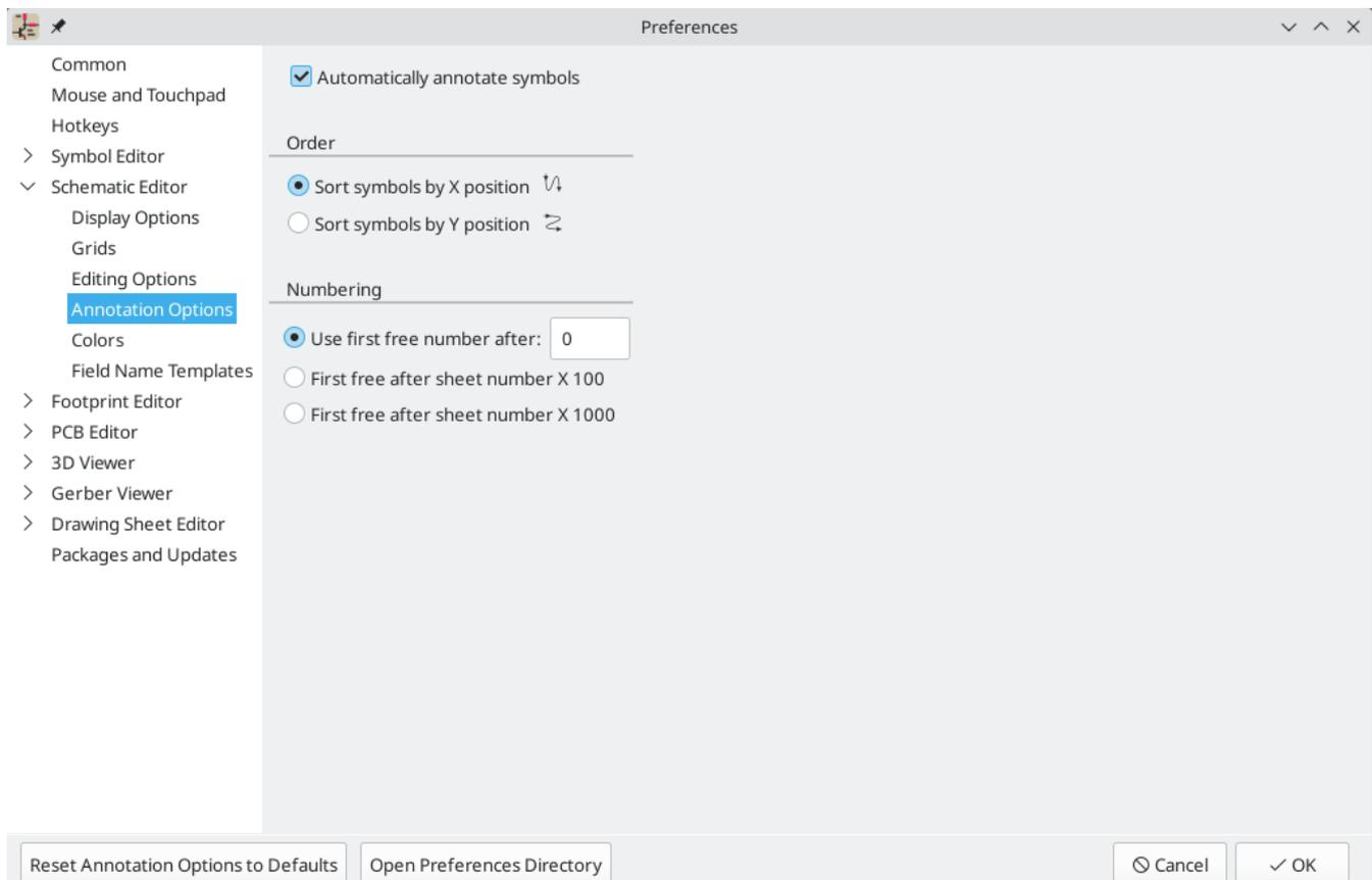
When multiple symbols are added simultaneously, they are annotated according to the **Order** setting, sorted by either X or Y position.
