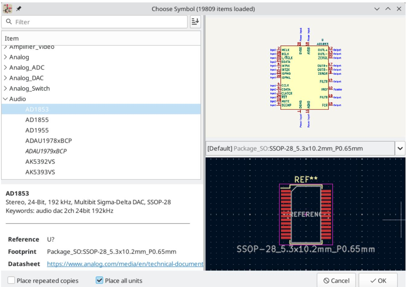
Symbols can have footprint filters that specify which footprints are appropriate to use with that symbol. If footprint filters are defined for the selected symbol, all footprints that match the footprint filters will appear as options in the footprint dropdown. The selected footprint will be displayed in the preview canvas and will be assigned to the symbol when the symbol is added to the schematic.
