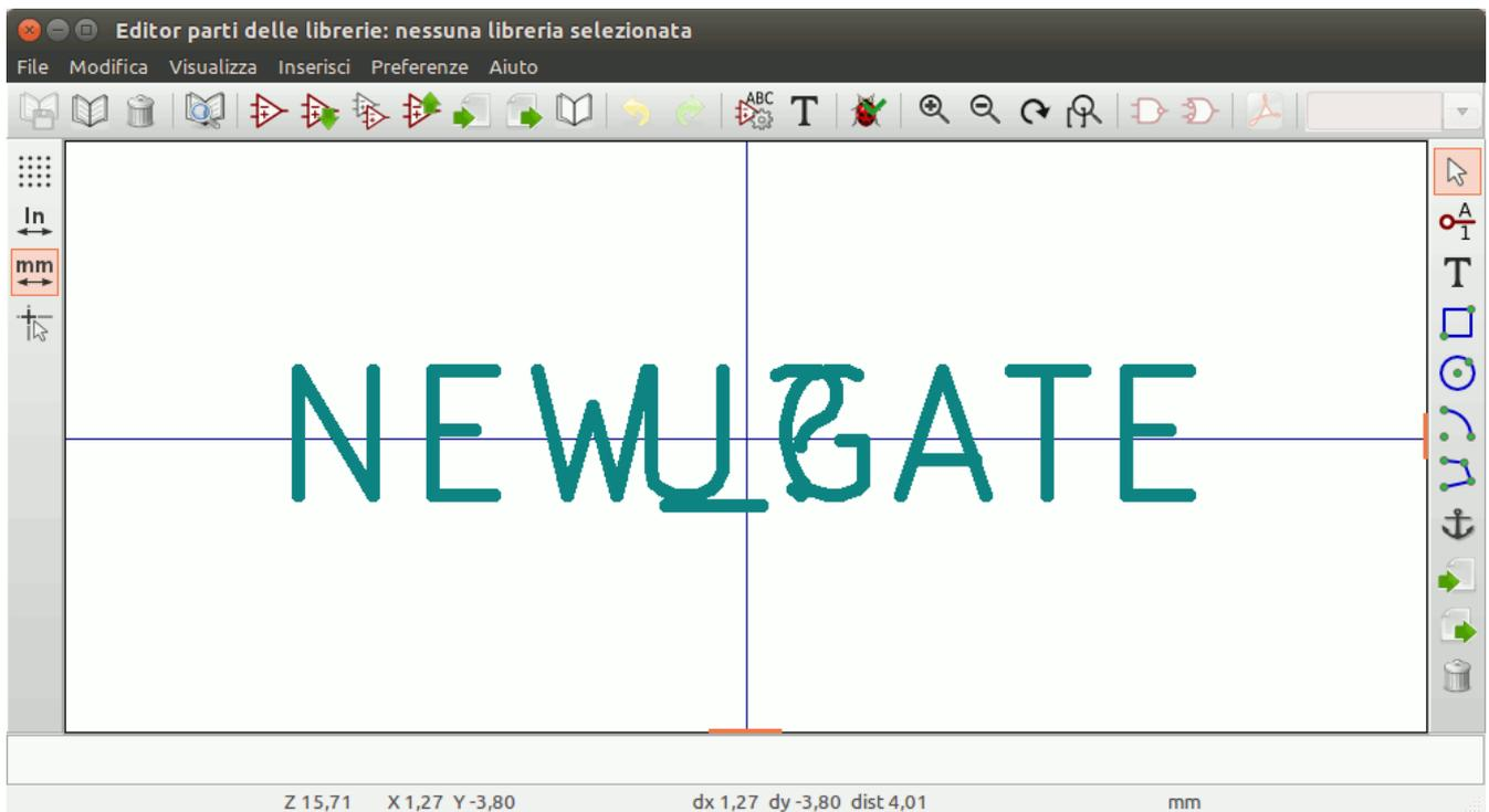
The blue cross in the center is the symbol anchor, which specifies the symbol origin i.e. the coordinates (0, 0). The anchor can be repositioned by selecting the
