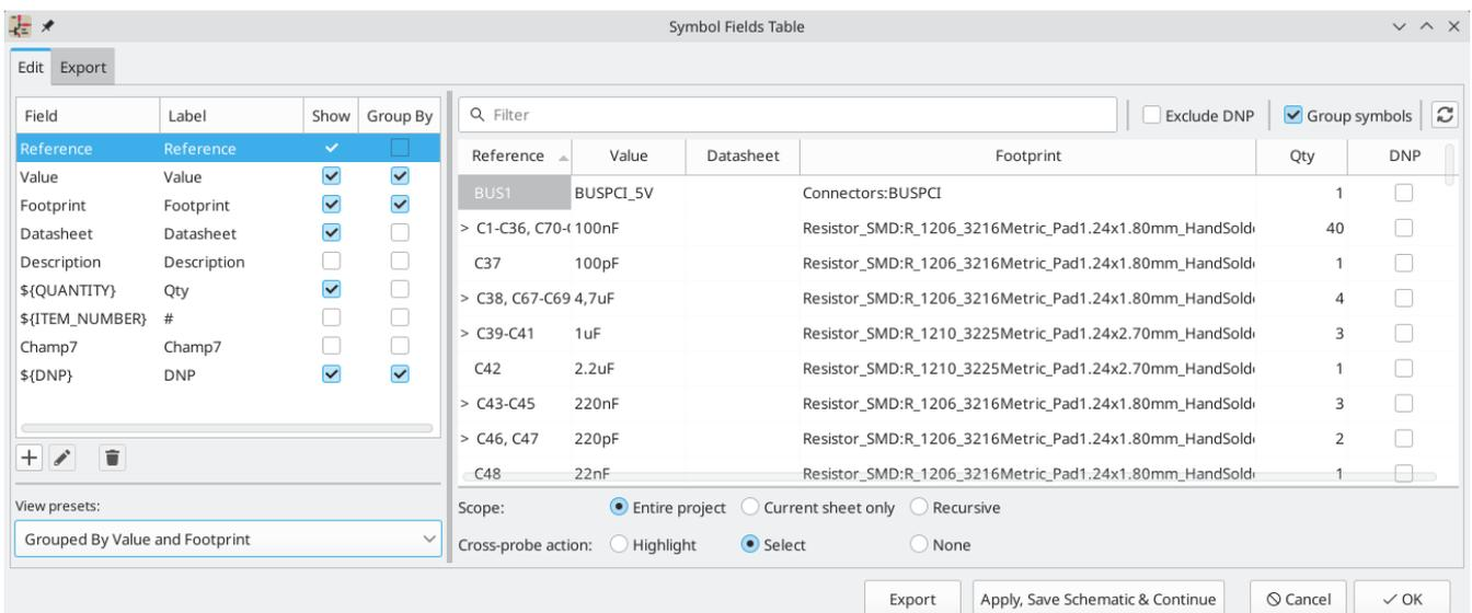
Fields with the **Show** box checked will be included as columns in the BOM, and fields with the **Group By** box checked are used to group components together. Components are grouped into the same line if all of their **Group By** fields are identical and the **Group symbols** box is checked. You can set an arbitrary column name for each field and reorder columns by dragging their headers.
