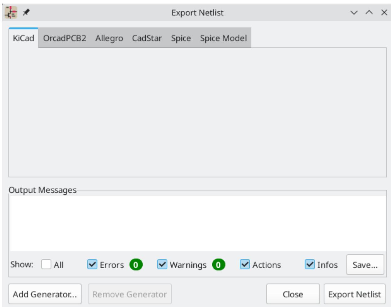
KiCad supports exporting netlists in several formats: KiCad, OrcadPCB2, CADSTAR, Spice, and Spice Model. Each format can be selected by selecting the corresponding tab at the top of the window. Some netlist formats have additional options.
