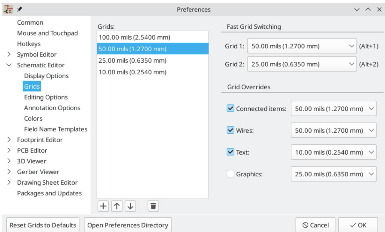
In this dialog you can select an active grid from the list of grids, reorder the list of grids, and add or remove grids. Grids defined in this dialog can have unequal X and Y spacing as well as an optional name.
