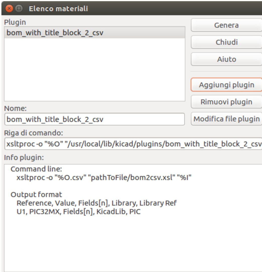
Several BOM generator scripts are included with KiCad, and users can also create their own. BOM generator scripts generally use Python or XSLT, but other tools can be used as long as you can specify a [command line](#) for KiCad to execute when running the generator.
