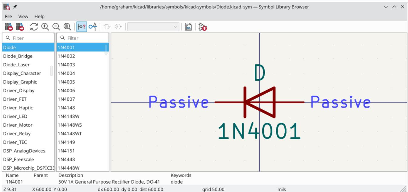
Double clicking the name of a symbol or using the
