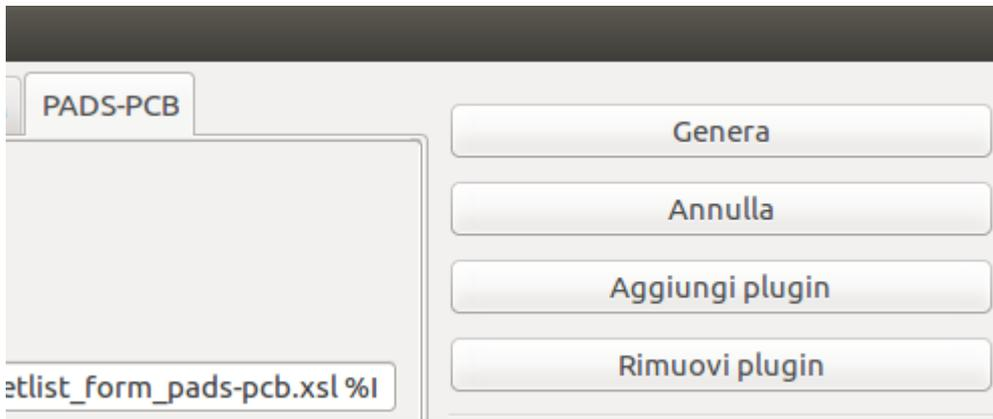
New generators require a name and a command. The name is shown in the tab label, and the command is run whenever the **Export Netlist** button is clicked.
