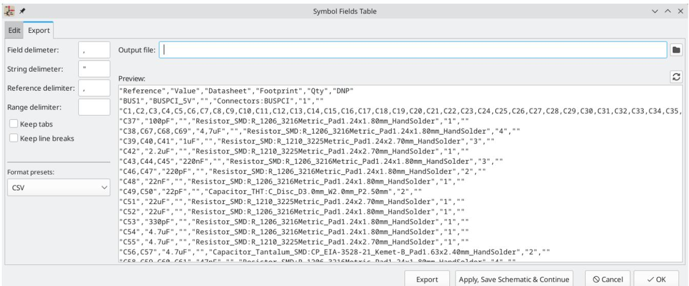
At the top you can specify the output file. Pressing the **Export** button will write the BOM to this file path. This path can contain [text variables](#).
