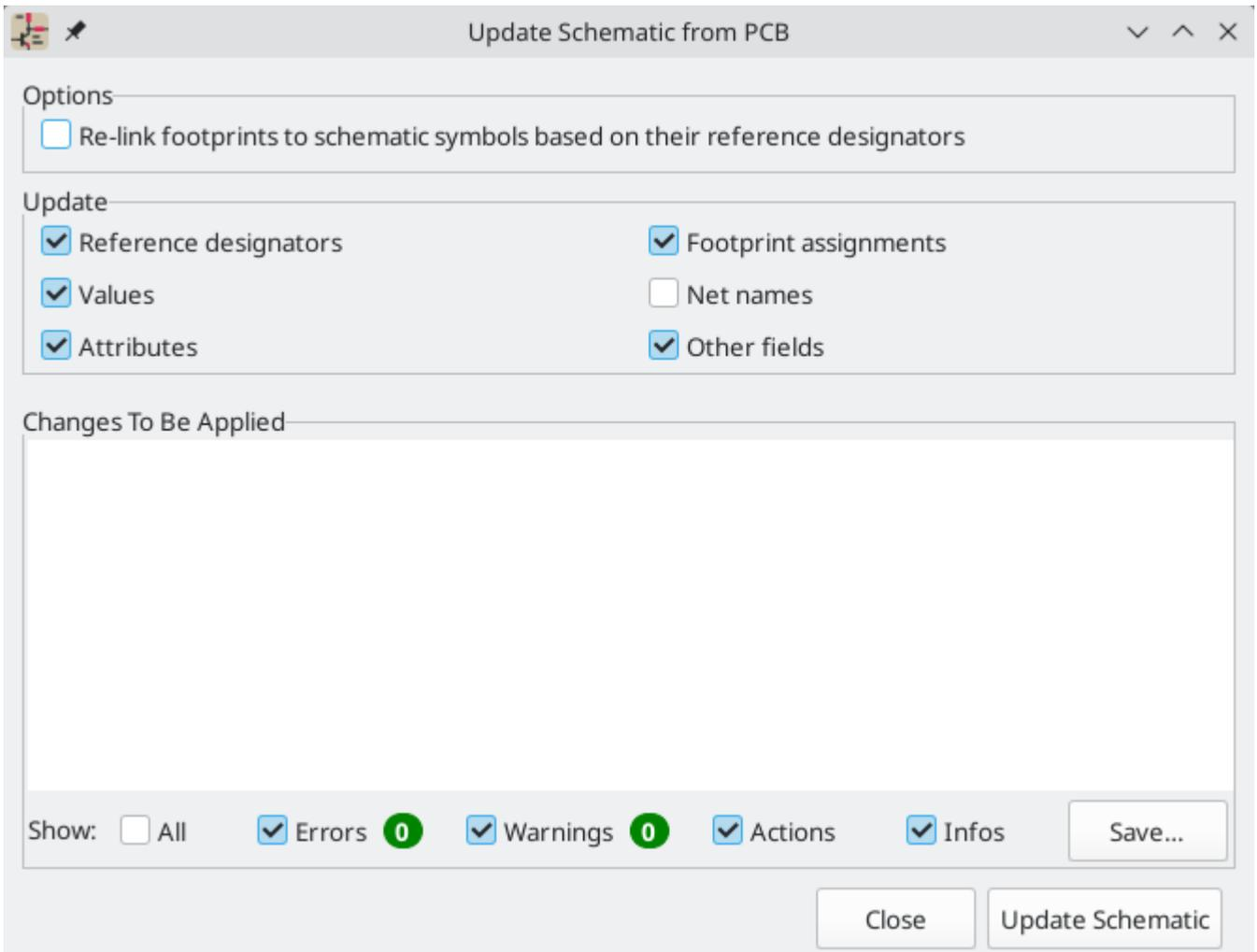
The tool syncs changes in reference designators, values, attributes (like DNP or Exclude From BOM), footprint assignments, other fields, and net names from the board to the schematic. Each type of change can be individually enabled or disabled.
