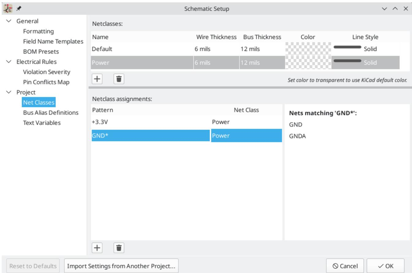
The top pane lists the netclasses that exist in the design. The `Default` netclass always exists, and you can add additional netclasses with the **+** button or remove the selected netclass with the **🗑** button.
