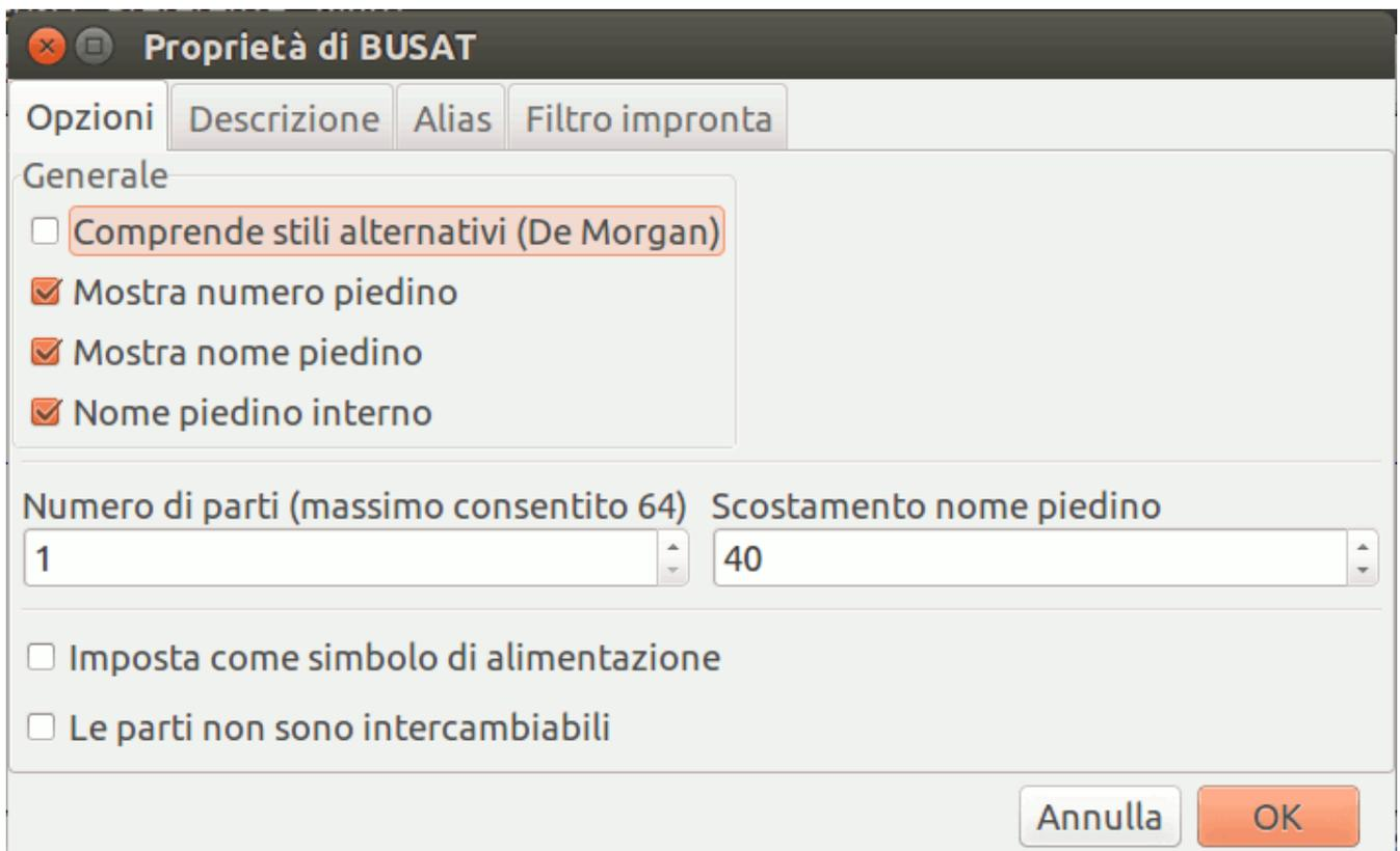
It is important to set the **number of units** and check **all units are interchangeable** and **has alternate body style**, as applicable, because these settings affect how pins and graphics are added to each symbol unit.
